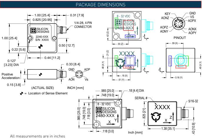
Contact SDI for data sheets pertaining to 2240s with serial numbers below 3000 and 2480s with serial numbers below 195.
